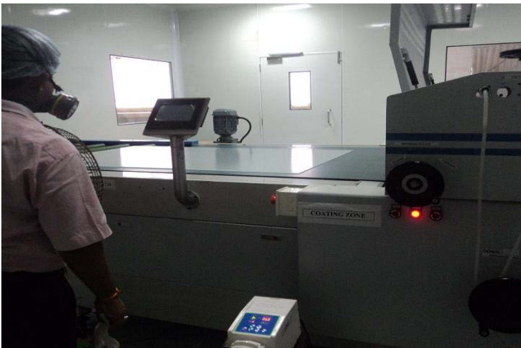
AR COATING PROCESS IN A CLEAN ROOM
