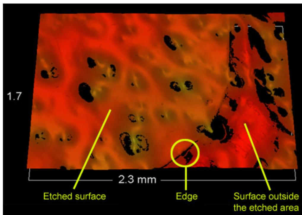
Figure 3. The surface of the glass after etching. The picture shows a faint edge from the Teflon spacer in the SAC. The glass surface is much more uneven than that of ordinary float glass.
