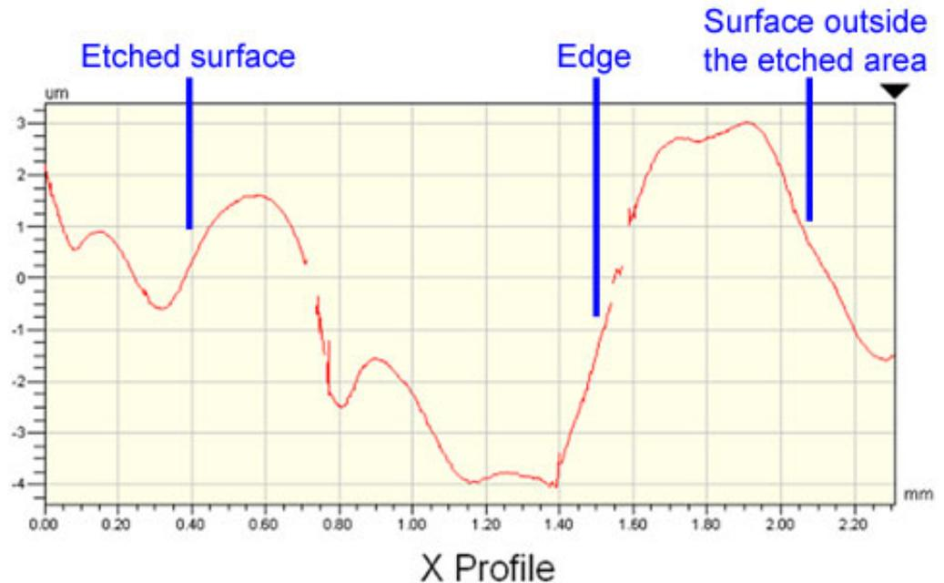
Figure 4. The surface of the glass after etching. From the X-profile, the height of the edge can be estimated as 7 micrometer. The glass surface is much more uneven than that of ordinary float glass.
